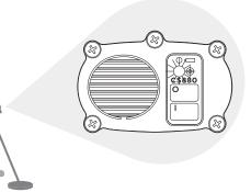
Detection of a metal cover is indicated by an audible pitch increase and target light brightness increase. Small metal targets are ignored.
