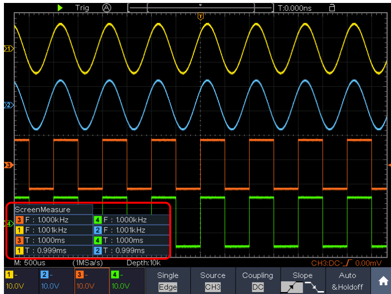
Figure 8-1 Measure period and frequency value for a given signal
