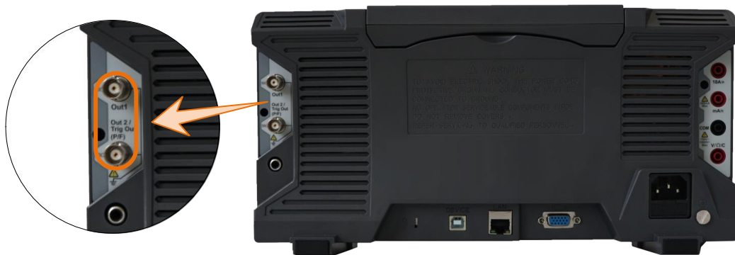
Figure 5-1 Generator Output Ports (Dual-channel)
