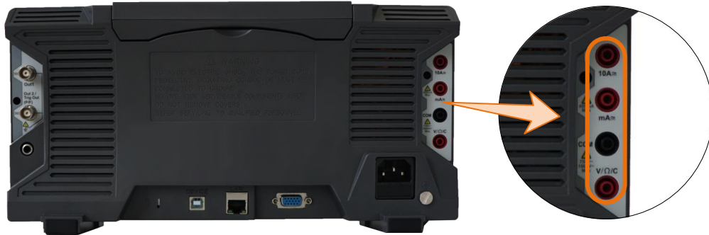
Figure 5-1 Multimeter Input Terminals
