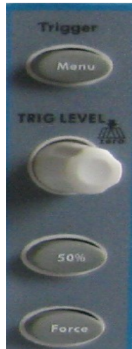
Figure 4-14 Trigger Control Zone
