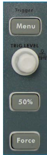
Figure 3-13 Trigger Control Zone
