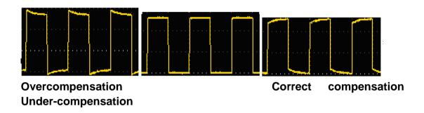
Figure 0-2: Display Waveform of Probe Compensation
