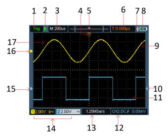
Figure 5: Oscilloscope Interface
